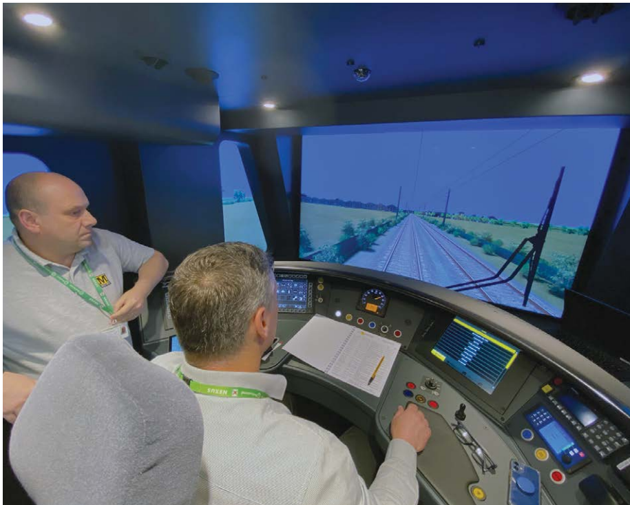
▲ To prepare drivers for the incoming Stadler trains, a new driver simulator has been installed at Nexus' Learning Centre in South Shields.
