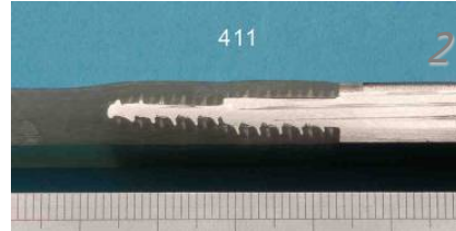
SS/GFRP joint made by vacuum infusion
