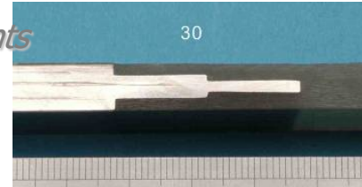
SS/GFRP joint made by vacuum infusion
