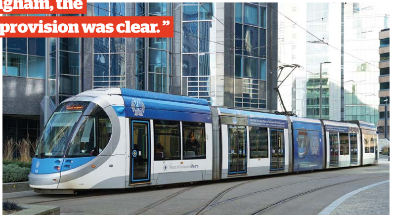
➤ RIGHT: Retrofitted with roof-top traction batteries, tram 19 is on Bull Street on 20 January 2020. The temporary livery commemorated the system’s 20th anniversary.
