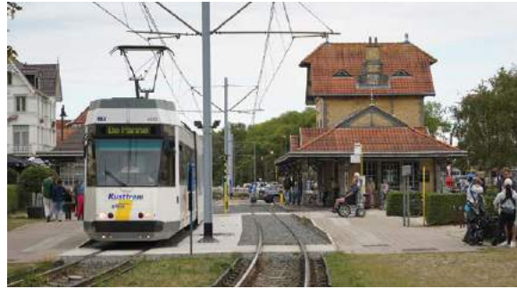
▲ ABOVE: The 1903 De Haan aan Zee (Coq sur Mer) station building now provides tourist information. The raised platform section aligned with the BN stock low-floor centre section; the right foreground was formerly occupied by a stub siding. Neil Pulling
