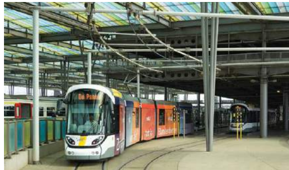
▲ ABOVE: Rebuilding Oostende's railway terminus reduced the distance needed for tram to train transfers. The layout allows for through services and for turning tram stock. Neil Pulling
