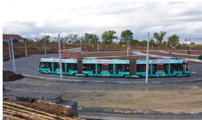
▲ The new loop at Slivenec is particularly large and wide, taking advantage of its peripheral location on a former greenfield site that awaits development. One day after the opening of the newest tramway extension in the Czech capital, Škoda 15T LRV 9377 waits with a line 5 service on 14 October 2023. A. Thompson
