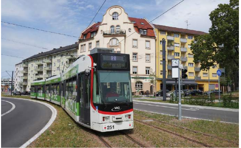
▲ ABOVE: Duewag GT8Z 251 is at Kaiserstuhlplatz , where the new alignment onto Waldkircher Strasse diverges from the route through Komturstrasse . The new tracks are framed by greenery and run on reserved formation.
