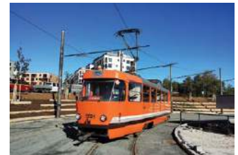
▲ ABOVE: Tatra T3S521, converted to a track and overhead catenary monitoring tram, undertakes trial runs on 17 October. DPP
