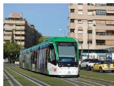
◀ LEFT: Artificial grass is widely used across the system, as on this wire-free section on Avenida de la Constitución between Caleta and Villarejo.
