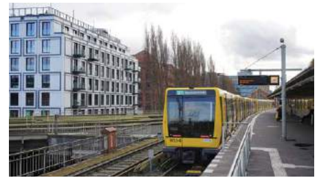
▲ ABOVE: The newest vehicles on Berlin's underground network are the narrow profile type IK . These have been locally produced by Stadler at its Pankow plant from 2015-20, with 54 such trains delivered in four separate series. In February 2023, 1053 is seen at the overground terminus of lines U1 and U3 at the major interchange Warschauer Strasse.
