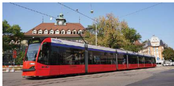
▲ ABOVE: Combino 761 is one of 15 low-floor, five-section Class Be 4/6 LRVs, which Siemens delivered in 2002-4. In 2009, eight were lengthened to become seven-section type Be 6/8 . In September 2020, the extended Combino 761 passes along Viktoriaplatz with an inbound line 9 service. To the right is the namesake Viktoriastrasse.
