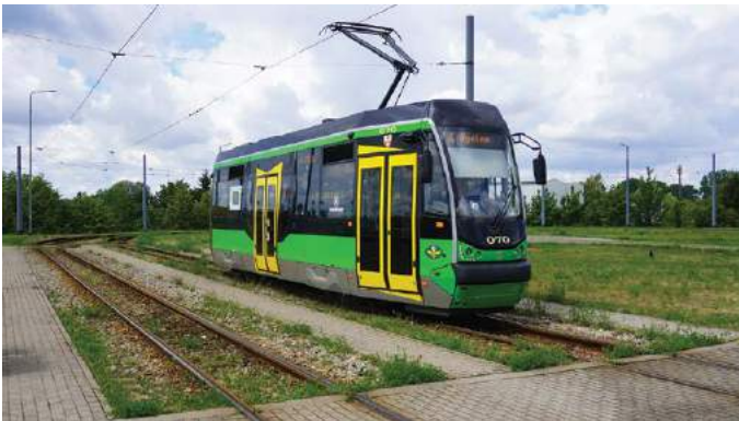
▲ ABOVE: The single-ended Moderus Beta MF 09 AC 070 idles at the Druska double-track turning loop, which is served by lines 1, 2 and 4 and is the southernmost point of the city's tram network. The low-floor centre section is visibly outlined by the vehicle's clever colour pattern.
