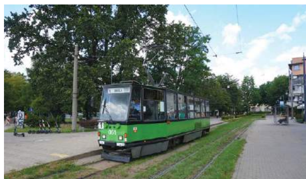
◀ LEFT: Car O61 is one of the non-modernised Konstals and still has printed destination boards rather than electronic dot-matrix displays. While running southbound on line 1 to Druska, the single-ended tram calls at Plac Grunwaldzki. Due to their angular design and large panel windows, these still ubiquitous trams are known as 'Aquariums' all over Poland.
