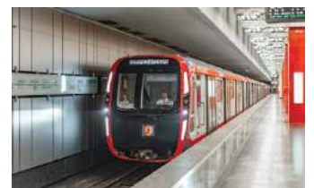
▲ An 891-775 (Moskva 2020) train on the metro at Michurinski Prospekt on the extension of Line 8A, which opened in 2018. Over 200 of these trains are now in service. S. Gvozdi
