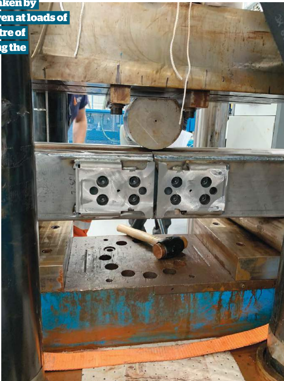
▼ BELOW: Junction plates being tested at British Steel.
