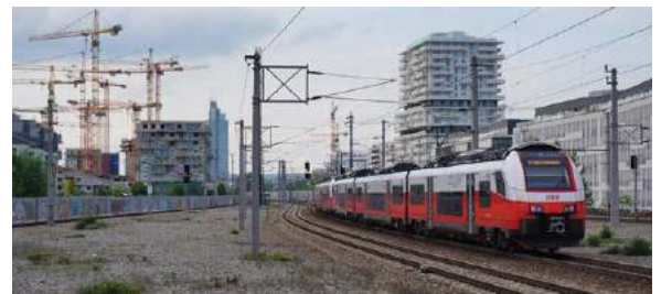
▲ ABOVE: Vienna's S-Bahn commuter railway is operated by the state railway company ÖBB using a variety of single-deck and double-deck trains. Pictured here are two coupled sets of the newer Class 4746 Siemens-built CityJet EMUs on their approach to Wien Praterstern. Development of the system started in the early 1960s and currently ten lines are in operation. The core section is the 11.3km (seven-mile) Stammstrecke (trunk route) from Wien Meidling to Wien Floridsdorf via Wien Hauptbahnhof, Wien Mitte and Wien Praterstern. The centrepiece of the S-Bahn trunk route is formed by several underground tunnel sections between Wien Hauptbahnhof and Wien Radetzykplatz. Around 640 trains and over 270 000 passengers travel on S-Bahn trains over this core artery every day.
