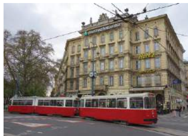
▲ ABOVE: The Duewag type E2 articulated trams haul type C5 bogie trailers in order to provide sufficient capacity. Here, car 4324 and trailer 1473 have just turned onto Ringstrasse and are now running on line D towards the Opera.
