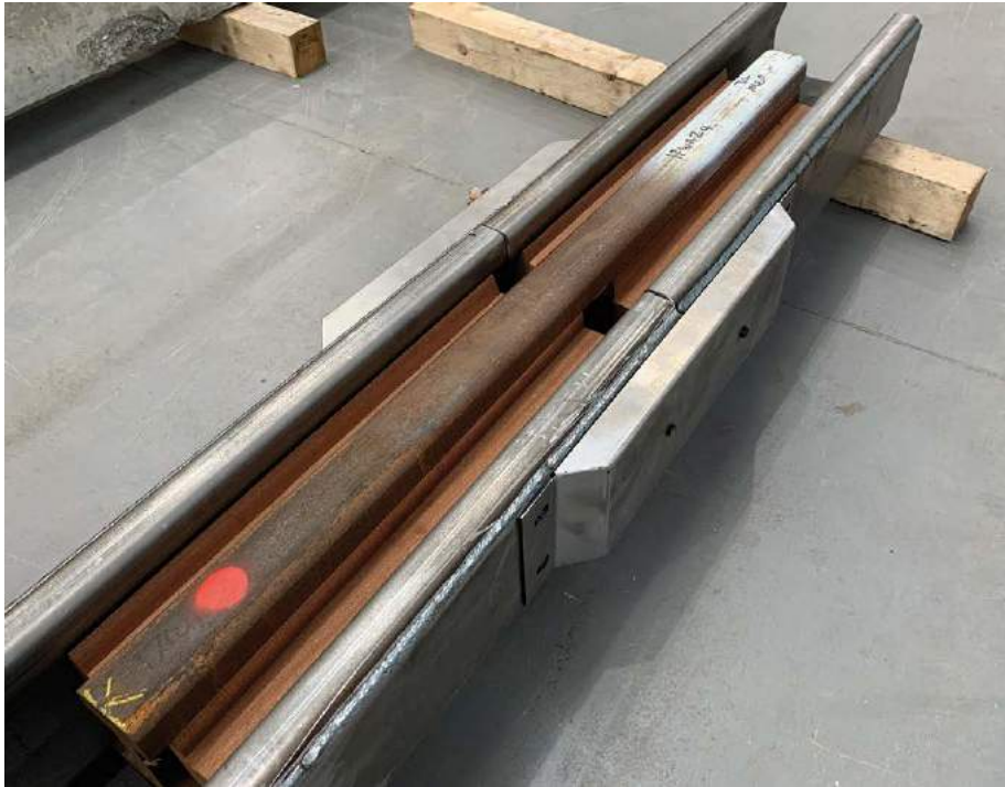
▼ BELOW: Full assembly of trackform with blocks and junction plates fitted.
