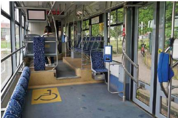
▲ ABOVE: Apart from a prototype in Ostrava, Košice is the sole operator of the TW Team Vario LF2+ . The two low-level areas approximate to 43% of the total.
