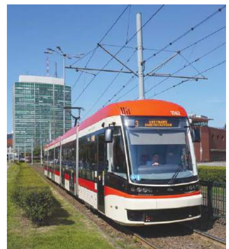
▲ ABOVE: Double-ended Pesa Jazz car 1062 on the approach to the central interchange at the main railway station.
