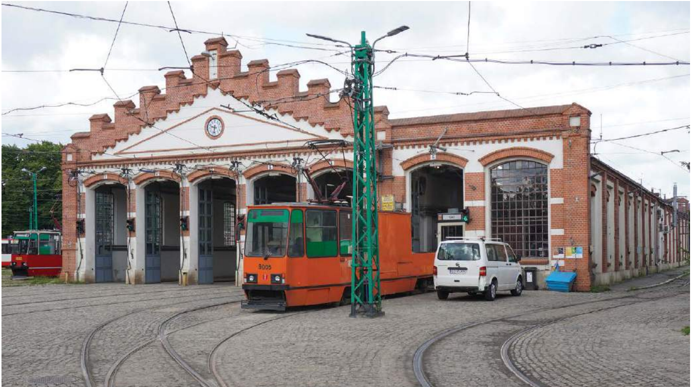
▲ ABOVE: Konstal car 9005 outside the historic Nowy Port depot building. This specially modified tram is used for infrastructure maintenance.
