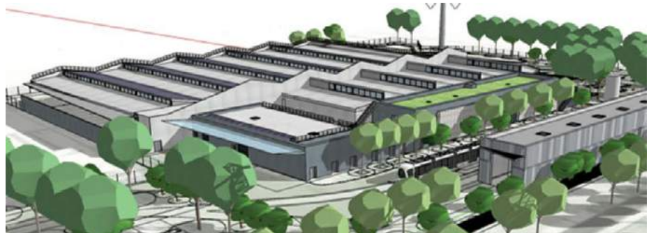
◀ LEFT/ ABOVE: The Saint-Fons maintenance centre uses solar thermal energy to supply its domestic hot water, and produces its own electricity via photovoltaic solar panels. Systra
