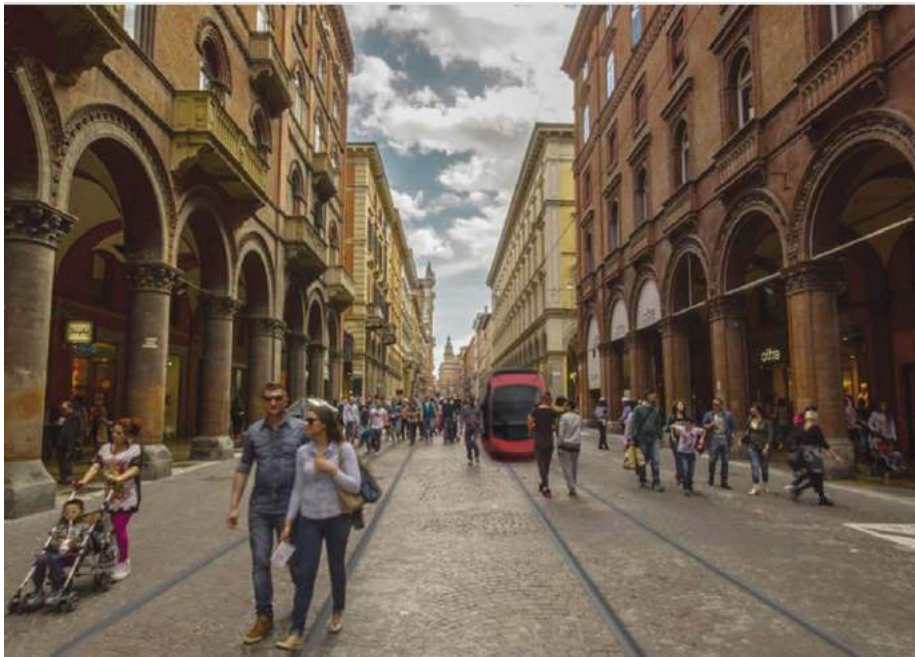
▲ ABOVE: The centre of the city is the most sensitive from a historical perspective; the tramway will run on a 2km catenary-free system using batteries. Catenary will run along the remainder of the line, with the poles integrated into street lighting.
