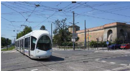
▲ ABOVE: Running on T6, which was launched in November 2019, Citadis 47 approaches the diamond junction at Desgenettes, where the tracks of line T6 cross T4 at a right angle. The curve to the left is only used as a possible diversionary option. T6 is now slated for another 5.4km (3.4-mile) extension further north, which will take the line to the university campus by 2026 and is expected to see ridership increase to 55 000 a day. The EUR176m project is expected to be completed by 2026, together with the construction of the new orbital lines T9 in the northeast and T10 in the south.
