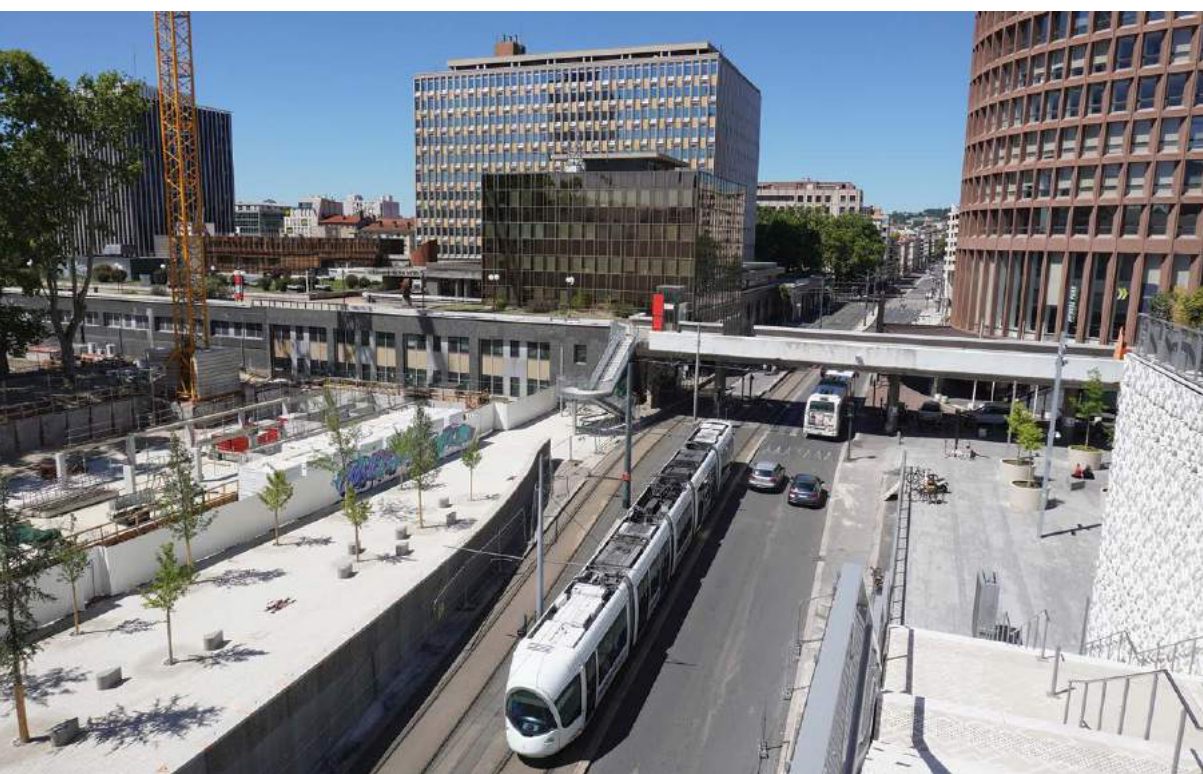
▲ ABOVE: Running on T6, which was launched in November 2019, Citadis 47 approaches the diamond junction at Desgenettes, where the tracks of line T6 cross T4 at a right angle. The curve to the left is only used as a possible diversionary option. T6 is now slated for another 5.4km (3.4-mile) extension further north, which will take the line to the university campus by 2026 and is expected to see ridership increase to 55 000 a day. The EUR176m project is expected to be completed by 2026, together with the construction of the new orbital lines T9 in the northeast and T10 in the south.
