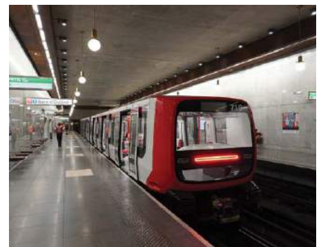
▶ RIGHT: Just a few days after metro line B was switched to driverless operation in late June 2022, the new Alstom Urbalis two-coach unit 719 stands at the southern line B terminus Gare d'Oullins. Instead of using a glass enclosure with automatically opening doors, line B is fitted with optical infrared sensors near the platform edge, just like Lyon metro line D.
