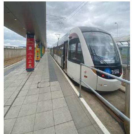
▲ ABOVE: Edinburgh Trams uses a fleet of 27 CAF Urbos 3. More trams are likely to be required for the future North South Tram project.
