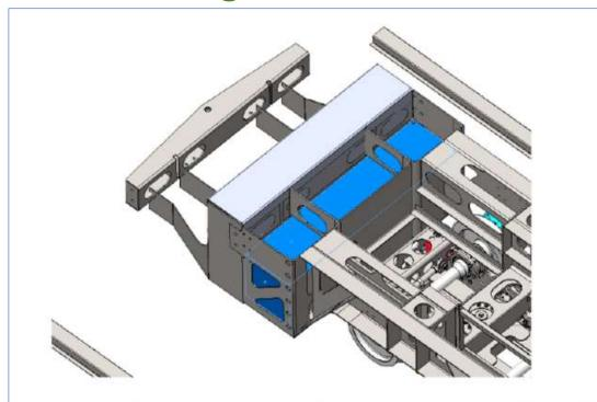
View of battery compartment with Li-ion battery pack highlighted (blue)
